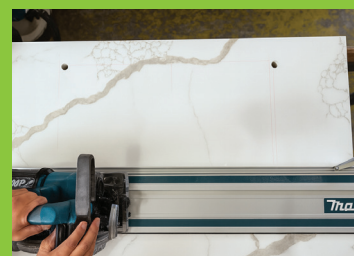
Use woodworking tools for cut-to-size and installation
